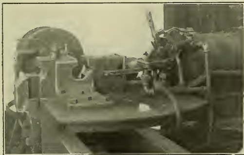
Flue Swedge Used on the Oregon Short Line.
